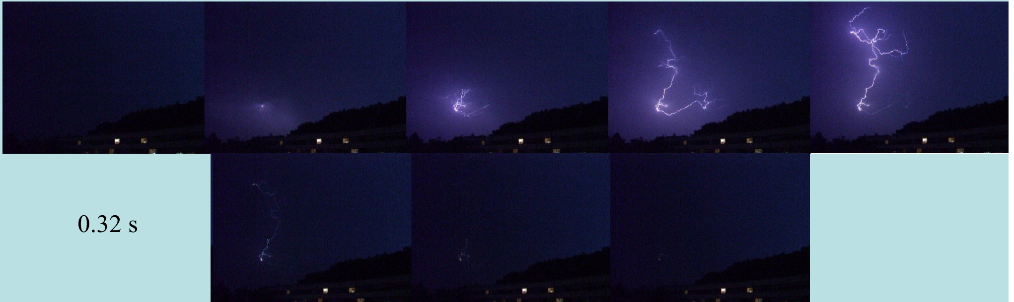
High-speed photography showing different parts of a lightning flash during the discharge process as seen in Toulouse, France.
