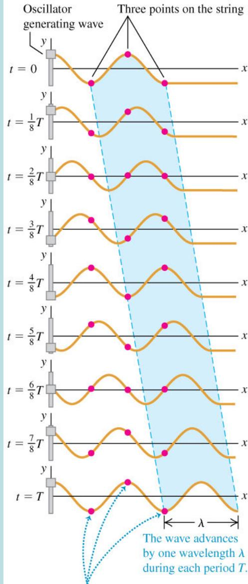
Each point moves up and down in place. Particles one wavelength apart move in phase with each other.
