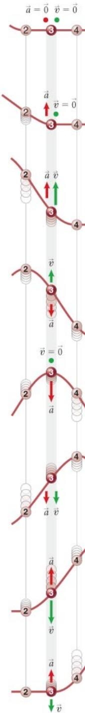
There can be a net vertical force on the segment, but the net horizontal force is zero (the motion is transverse).
