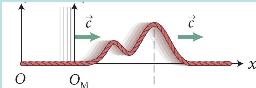
$$\frac{\partial^2 y}{\partial x^2} = \frac{\mu}{\tau} \frac{\partial^2 y}{\partial t^2} \quad \text{波方程式}$$
