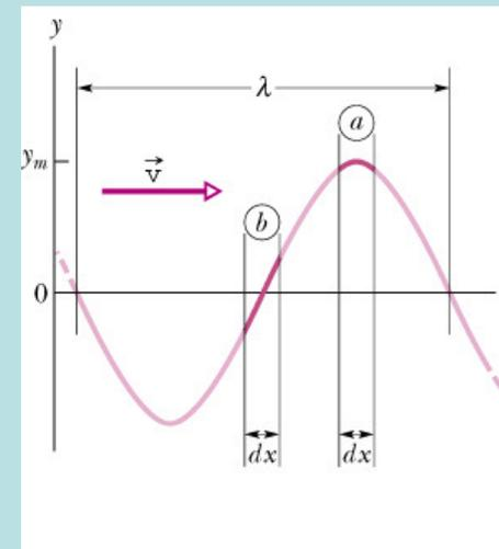
$$\text{動能密度} = \frac{\frac{1}{2}(\mu \Delta x) \left( \frac{\partial y}{\partial t} \right)^2}{\Delta x} = \frac{1}{2} \mu \left( \frac{\partial y}{\partial t} \right)^2$$
