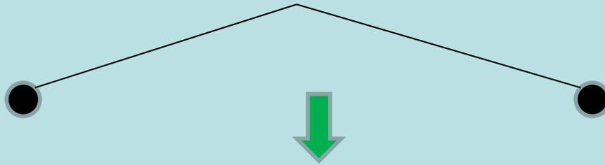
$$y(x, t) = \sin \frac{\pi}{L} x \cos \omega_1 t - \frac{1}{9} \sin \frac{3\pi}{L} x \cos \omega_3 t + \dots$$
