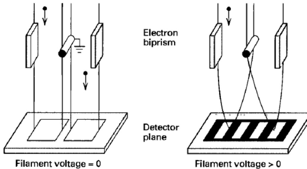
**Figure 1-7** (a) When the filament is grounded, the electrons passing one by one can be seen on the monitor, and the path can be identified. The shadow of the filament can be seen after many electrons have passed. (b) When a positive voltage is applied to the filament, the electrons are bent toward the center, and there is no way of telling which side of the filament the electron passed by. An interference pattern results.
