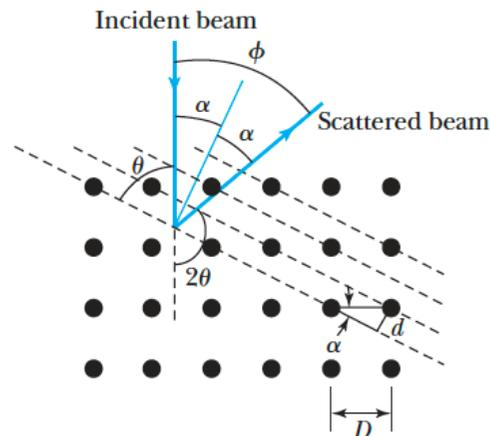
**Figure 5.11** The scattering of electrons by lattice planes in a crystal. This figure is useful to compare the scattering relations  $n\lambda = 2d \sin \theta$  and  $n\lambda = D \sin \phi$  where  $\theta$  and  $\phi$  are the angles shown,  $D$  = interatomic spacing, and  $d$  = lattice plane spacing.
