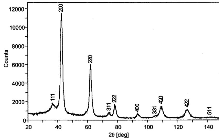
Fig. 1: X-ray diffraction of powder MgO (G. Dercz et al., Materials Science-Poland, 27, 1, 2009)
