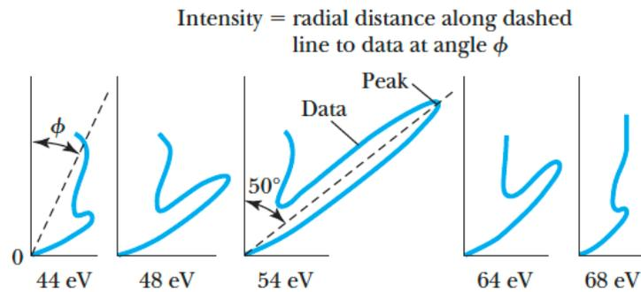
**Figure 5.10** Davisson and Germer data for scattering of electrons from Ni. The peak  $\phi = 50^\circ$  builds dramatically as the energy of the electron nears 54 eV. From C. J. Davisson, *Franklin Institute Journal* 205, 597–623 (1928).
