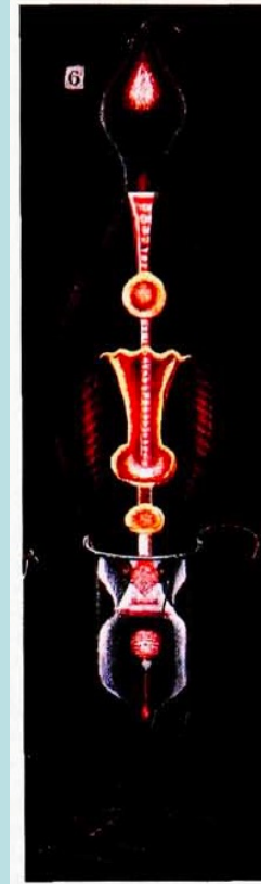
ELECTROLUMINESCENCE from this Gassiot cascade delighted and mystified 19th century audiences. The cascade consisted of a large goblet of uranium glass, lined with tin foil. When the goblet was placed on a metal plate, covered with a bell jar, and brought to the proper degree of evacuation, a machine for generating static electricity that was connected to the foil and plate caused, in the words of historian E. Newton Harvey, “spectacular electroluminescent effects . . . in the gas which seemed to flow over the edge of the goblet.” (Photo from the frontispiece to A. Privat Deschanel, Elementary Treatise on Natural Philosophy , vol. 3 [Blackie & Son, London, 1888].) FIGURE 3
