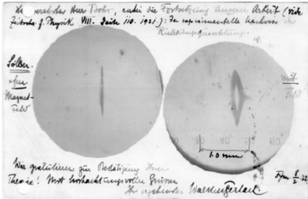
The postcard sent by Stern to Bohr showing the results of the Stern–Gerlach experiment. The left image shows the rectangular beam in the absence of the magnetic field gradient; the right-hand image shows the splitting of the beam into two components. The greatest field gradient occurs in the centre of the beam.
