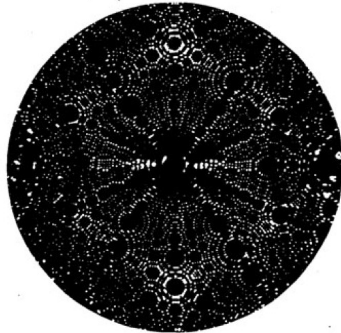
Figure 11.13. Field ion microscope image of a tungsten tip of radius \sim 400 \text{ \AA} . The original image had a magnification of 3 million. (Photo courtesy of T. Tsong.)
