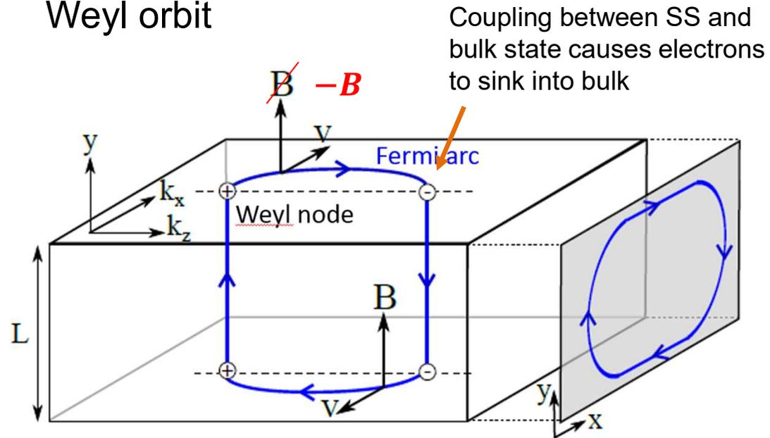
$$T = 2t_{arc} + 2t_{bulk}.$$
