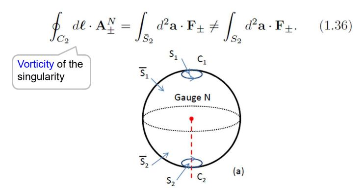
The LHS approaches  $2\pi$  as  $C_2$  shrinks to zero; while the last integral approaches 0. The inequalities arise because the Stokes theorem fails if **A** is singular in the domain of surface integration.
